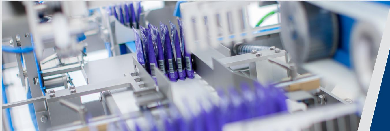
Our paddle chain was specifically developed to ensure efficient and gentle product handling, enabling precise product transfer and positioning at high speeds.
