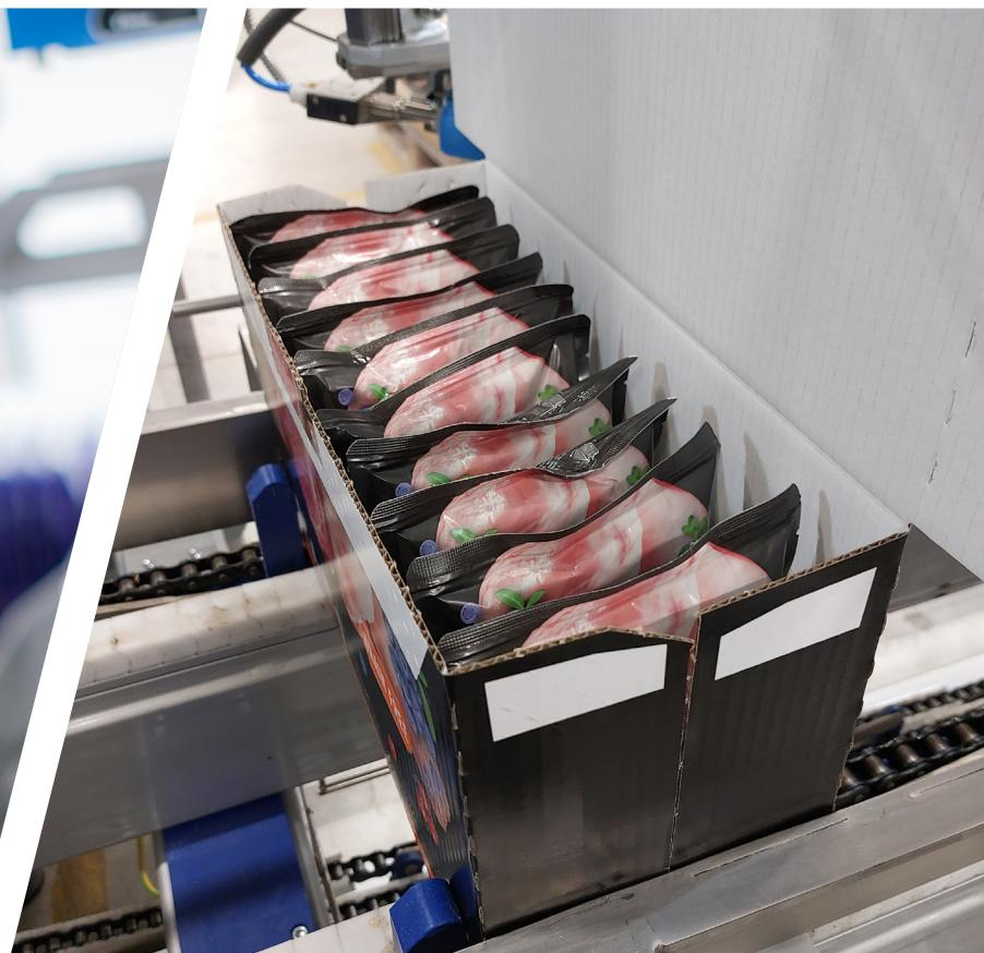
High-speed wrap-around case packer for up to 40 packaging units per minute. The modular design ensures efficient, reliable and flexible operation through simple format changes and optimal accessibility for maintenance. Specially designed for flexible primary packaging.
